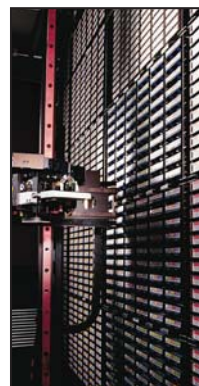
The Scalar 10K provides built-in room to grow, integrated SAN management, and dual redundant robotics.
